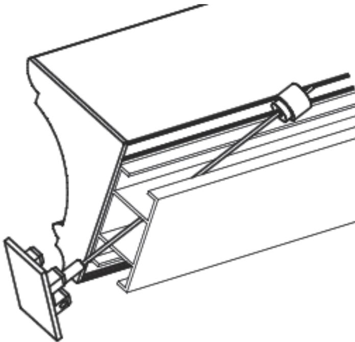
The Trim Maker extrusion and base are mounted to a Porsa extrusion. The graphic is inserted into spring clip holders. The spring clip holders are slid in through the end of the Porsa extrusion and the Porsa endcap is affixed. To change the graphic, remove the Porsa endcap, slide out the graphic and slide in the replacement.
