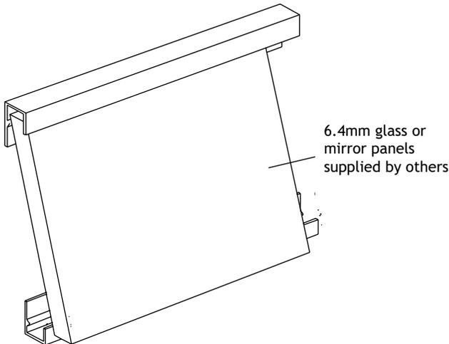
To install, simply position the mirror into the top channel, and then lower it into the bottom channel.
