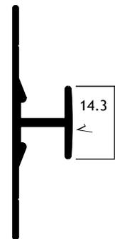
Divider trims are supplied slotted with holes for adjustability and rapid installation.
